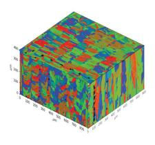
Building on Sentient's extensive history in computational modeling of crystalline material microstructures, the Microstructure Modeling feature of DC-AM leverages the thermal history computed during Process Modeling to predict the microstructure, including the grain structure and both lack-of-fusion and keyhole porosity, of parts built with AM.
