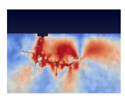
DC-E integrates Sentient's game-changing, proprietary approach to predicting onset of rolling contact fatigue and gear tooth bending fatigue based on microstructure-level models of damage initiation and early growth. Weibull analysis utilities are built into the software for easy results interpretation and comparison. This gives users a physics-based method to virtually assess the impact to reliability of choices of:
