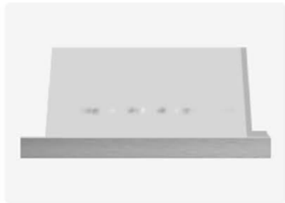
Damage Class 1 Minor Defect
