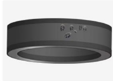
Damage Class 1 Minor Defect (Single or multiple spot micropitting or frosting observed within area of race)
