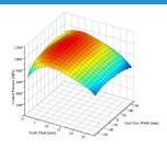
DC-E offers detailed contact and stress analysis capabilities for spur and helical gears, considering loading and microgeometry modifications to gear teeth to compute several key parameters relating to gear mesh interactions, including contact lines, contact pressure, surface velocities, static transmission error, and tooth root stresses.
