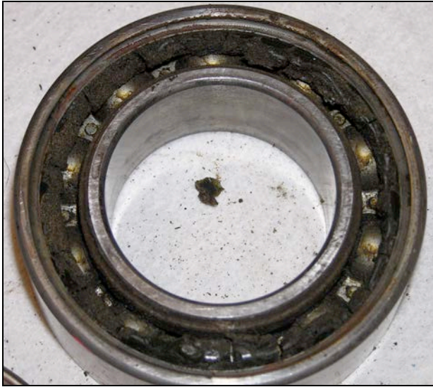
Figure 2: Debris-filled oil cooler bearing
