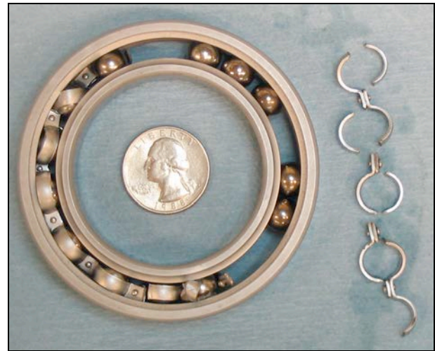
Figure 8: Degreased hanger bearing that seized in a lab test
