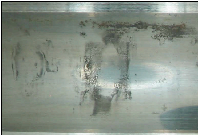
Figure 3: Oxidation of oil cooler bearing inner raceway
