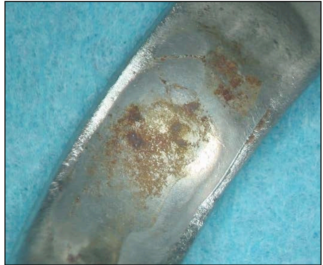
Figure 4: Corroded inner surface of the cage in the ball/cage contact region
